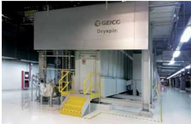
**The limestone-based Dryspin technology for extracting overspray paint from air extracted from the paintbooths, is a water-free process**
