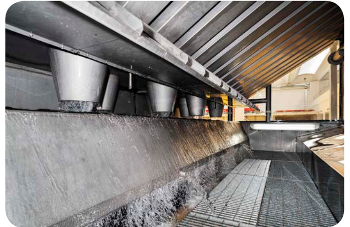
BELOW: Exhaust air is mixed with water in order to remove paint overspray particles generated in the painting booth during the painting process.
