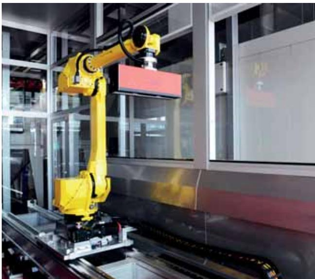
Geico believes Ctrl + PAINT is the first system operating independent of colour but is capable of detecting defects both topographical and non-topographical
