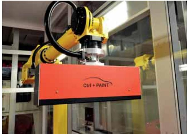
Ctrl + PAINT can produce the data needed to help identify the origins of a defect, and may be configured to automatically warn and adjust settings
