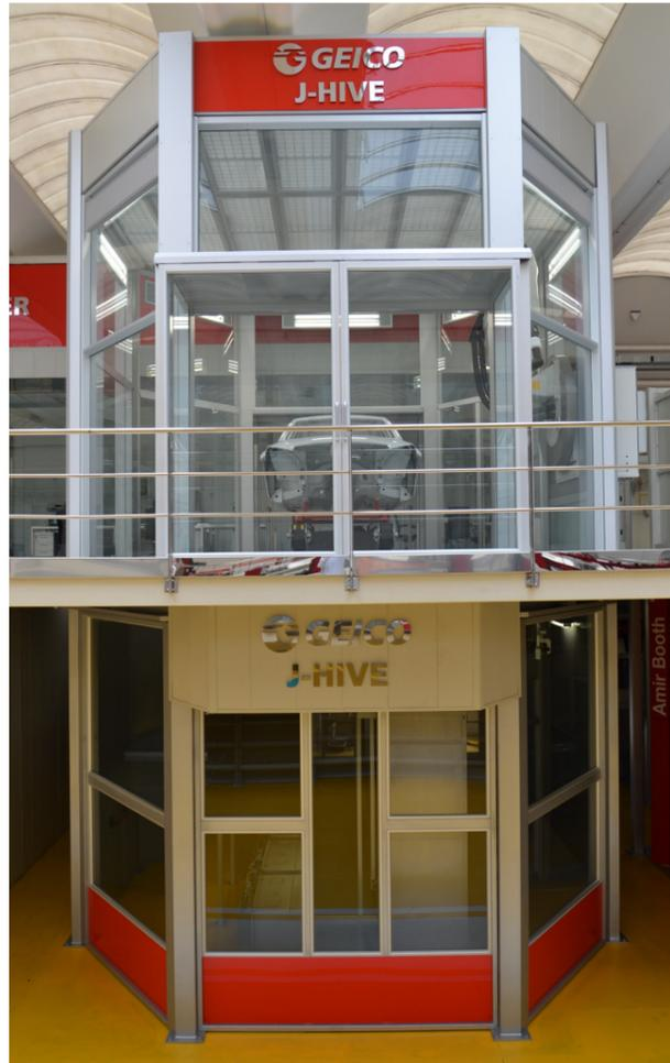
(Left) Customers can configure the octagonal J-Hive cells in a variety of ways (Right) The J-Hive cell allows several movements of the robot and the car body, reaching perfectly all internal and external surfaces
