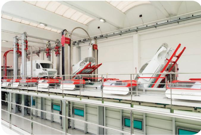
Immersing a body through rotation rather than dipping is one of the innovations that came out of Geico "Experiment Day".
